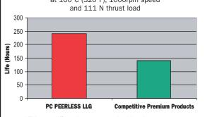
\* This test differentiates among wheel bearing greases having distinctly different high temperature characteristics. The longer the life, the better the protection.
