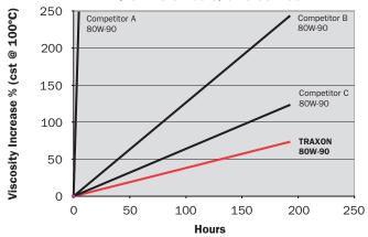
In the DKA oxidation test, product performance is measured by how much harmful viscosity increase will occur over time (therefore, the flatter the line the better). Compared to these competitors, Petro-Canada's TRAXON with its advanced formulation is clearly superior.
